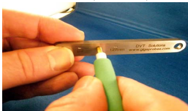
Fig. 3) Signal - Signal Pitch Calibration Wrench (patent pending) - Place the probe tips in the model 10 SMA calibration wrench to adjust S – S pitch to a fixed .8mm, 1mm, or 1.27mm spacing. Use the Desk-Top Macro-lenses Inspection Station to view probe tips and the precision Stainless Steel Tweezers for fine pitch adjustments.
