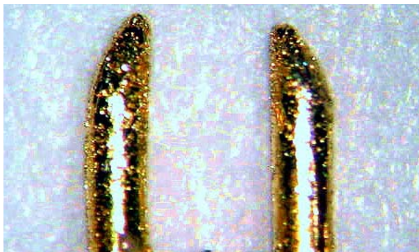
Fig. 4) Conductive Diamond & Gold Plated Tips (patent pending) – Hundreds of very sharp, non-oxidizing, conductive diamonds coat the probe tips easily break through surface oxide when probing, creating a connection as good as solder, allowing for repeatable TDR measurements and probing at any angle.
