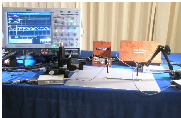
Fig. 6) Real-time Differential Impedance and S-parameters – Use two GigaProbes® to simultaneously extract differential impedance, insertion and return loss parameters to validate PCB interconnect impedance and bandwidth performance. Install GigaProbes® in manipulator for hand free measurements
