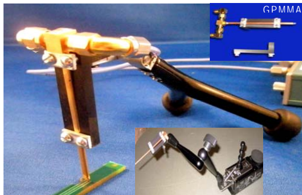
Fig. 2) Attaching GigaProbes® to Micro-positioners – The GPMMA adapter is a standard accuracy that attaches the Free-Hand Probe holder and the Ez-probe from LeCroy.
