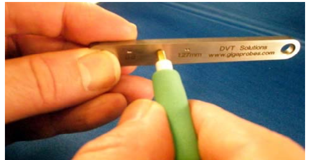
Fig. 3) Signal - Signal Pitch Calibration - Place the probe tips in the (patent pending) Model 10 SMA calibration wrench to adjust S – S pitch to a fixed 0.8 mm, 1.0 mm. or 1.27 mm spacing. Use the Desk-Top Macro-lens Inspection Station to view probe tips and the precision Stainless Steel Tweezers for fine pitch adjustments.
