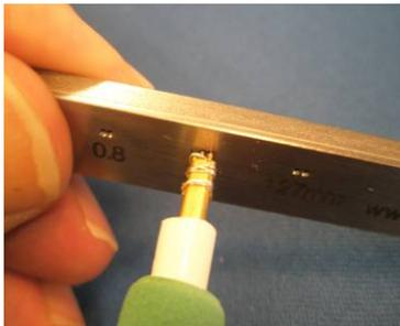
Push the probe tips into the 1mm holes in the GigaProbes™ patented pitch setting wrench. This will push the wire down flat against the probe body.
