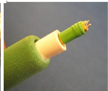
This is how it should look. Make sure the wires do not short the probe tips together.
