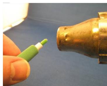
Use a heat gun to quickly shrink the tube tightly around the probe tip. **DO NOT OVER HEAT OR RISK DAMAGING PROBE**
