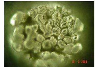
A Close-up view of a Diamond Partial Interconnect showing several sharp points that at as many probe tips in parallel reducing interconnect inductance. www.ditek.us.com
