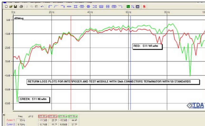
Return Loss for IC test board with Diamond Interpose shows 3dB enhancement with of high integrity contact even with Marginal PCB technology
