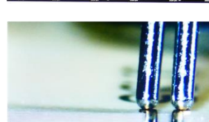
FPP70-0.60-001 SN 2083 Probe with 0.60 mm pitch probe tips
