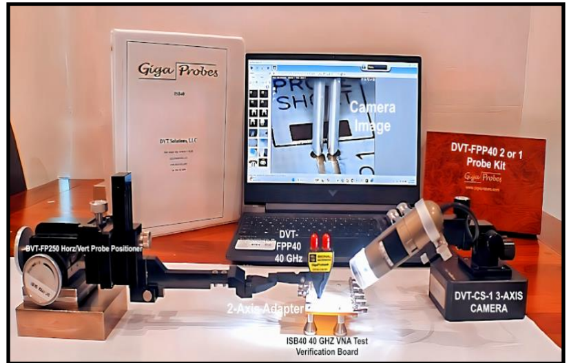
Figure 4. DVT-FPP40 probe system measuring the ISB40 probe-to-connector trace to verify probe de-embedding file accuracy.
