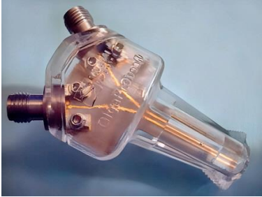
(2018 prototype) Differential PCB-based prototype probe design
