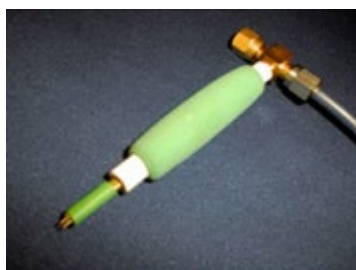
Attach a SMA SHORT CAP to the same probe, shorted to the probe body. Hook up your SMA Cable for a 50 Ohm TDR measurement
