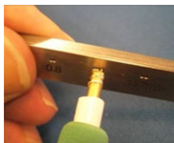
Push the probe tips into the 1mm holes in the GigaProbes™ patented pitch setting wrench which will push the wire down flat against the probe body.
