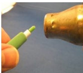
Use a heat gun to quickly shrink the tub tightly around the probe tip. DO NOT OVERHEAT OR YOU RISK DAMAGING THE PROBE!
