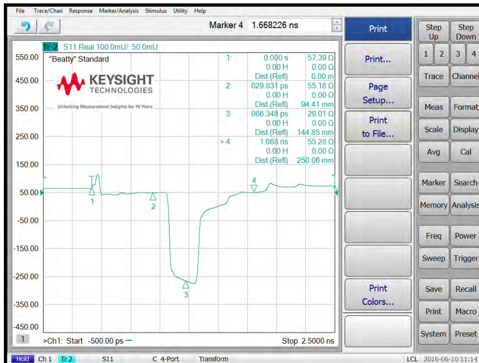
50/25/50 Ohm Beatty line Time Domain Plot to 50 GHz (DB50-002/003)
