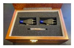
70 GHz Dual Probe Differential TDR and S-Parameters Probe kit. Contains two fixed differential probes. Includes a copper shorting block for creating probe models.
