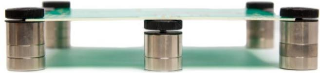
Use a DVT-SM Holder to secure each corner of a test board to keep it from moving while probing. Then remove one segment out of two additional holders and place them under the probing locations to keep thin test boards from bowing when probing. Fixture almost any size test board for horizontal probing applications. Four to six holders recommended.
