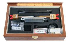
40 GHz/~4.5 ps Dual Probe Differential Multi-Mode TDR and S-Parameters Probe kit. Contains two variable pitch conductive diamond-plated DVT40 differential probes, convertible to 50 ohms. Includes pitch setting tools and four 17-inch 25 GHz cables.
