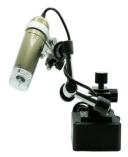
Camera System used to accurately place probe tips on test pads and to planarize the probe tips to the test pads so both probe tips land on the pads at the same time.
