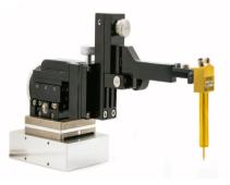
Rigid arm probe manipulator with XYZ pitch 40 TPI controls & magnetic base. Recommended for probing with DVT40 and DVT-FPPXX probes.
