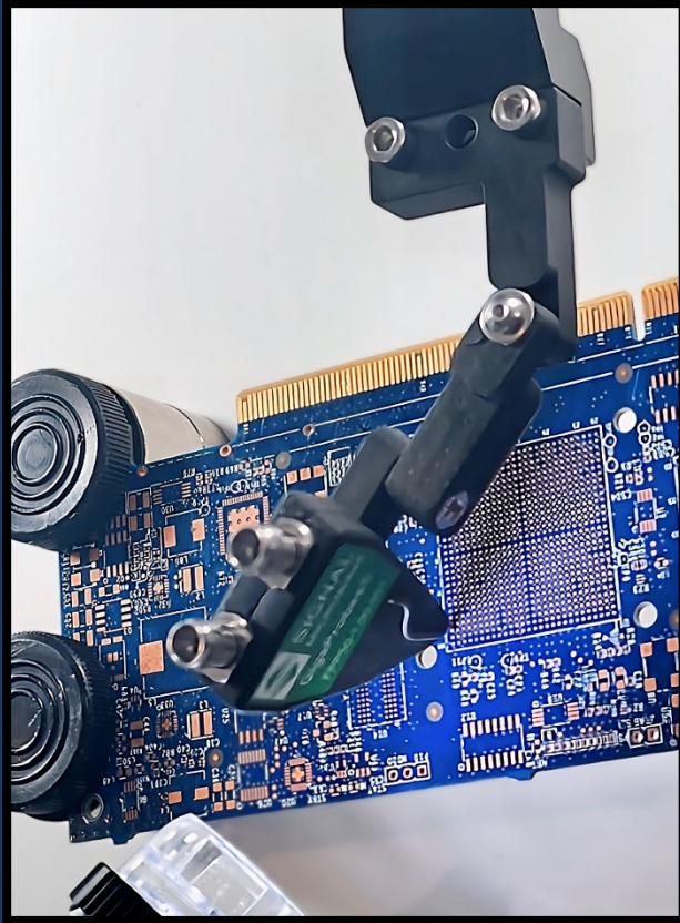
Horizontal probing: 45° oriented test pads on horizontal fixtured PCB - Probe can be on left/right side - Probe straight down
