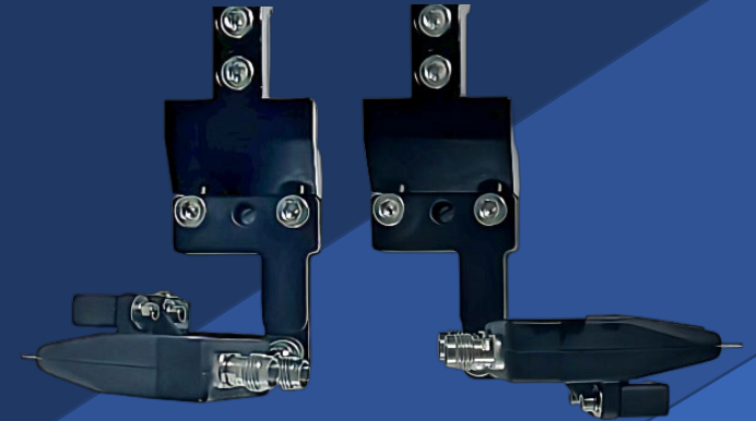
Vertical probing with arm 90° to a vertically fixtured PCB - Probe is lifted to contact vertically oriented test pads
