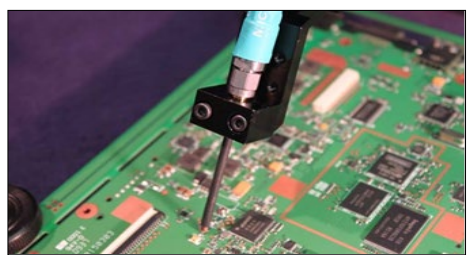
Single-Ended Fixed Pitch Probe System. The probe is attached to an adapter and to the end of a Probe Positioner arm. Several fixed pitches and bandwidths are available.
