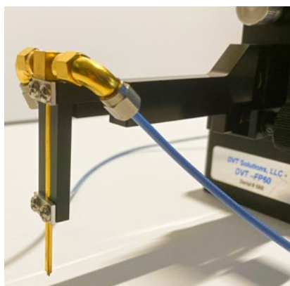
Fig 5. (Above left) DVT30 probe shown mounted in our GPPMA adapter and cables laying loosely on the table. (Above right) shows the DVT30 converted to a single ended probe. An SE conversion kit and instructions for conversion are included in the DVT30-1mm kit.
