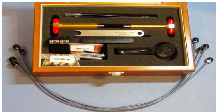
Fig 1. DVT30-1MM Dual Multi-Mode TDR kit: Two Differential (convertible to SE) probes, pitch adjustment tools and four 25GHz RF cables.
