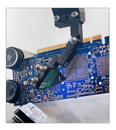
Horizontal probing: 45° oriented test pads on horizontal fixtured PCB
