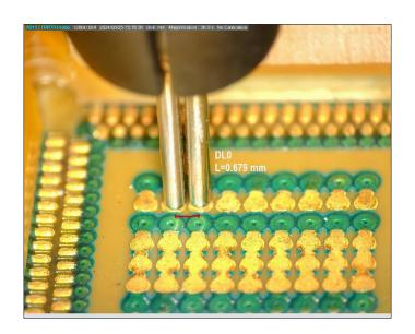
DVT-FPNN Differential rugged probe extends reach into test sockets or onto board-to-board interposers with force to make impedance and S-parameter bandwidth measurements to 70 GHz.
