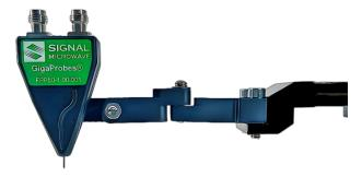
Horizontal Probing: Probe horizontally or vertically oriented test pads on horizontal fixtured PCB
