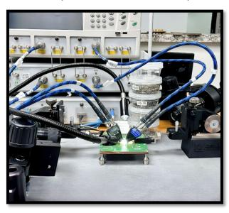
Probe tips are placed with 1 mm spacing.
