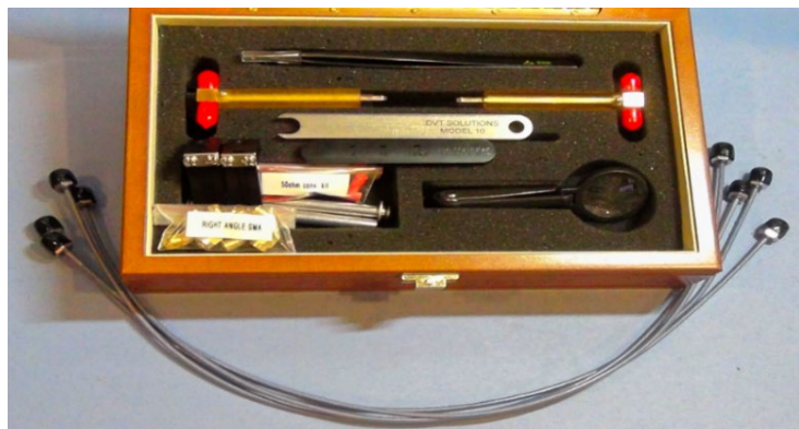
Fig 1. DVT30-1MM Dual Multi-Mode TDR kit: Two Differential (convertible to SE) probes, pitch adjustment tools and four 25GHz RF cables.
