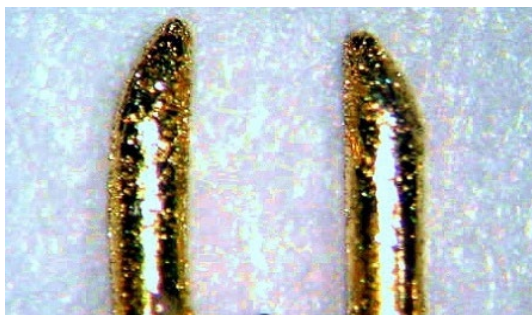
Fig 6. DVT30 probe tips plated with 4/6 \mu m conductive diamond that cuts through surface oxide for reliably repeatable measurements.
