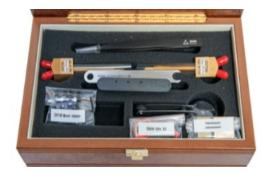
**Functionality**: 40 GHz/~4.5 ps Dual Probe Multi-Mode TDR & S-Parameters Probe kit.
