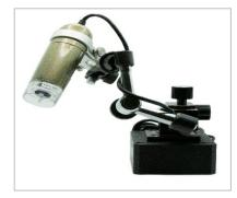
The Camera System is used for the accurate placement of probe tips on the test pads, probe tip planarization and calibration.
