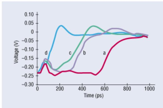
**Figure 10.** Superimposed waveforms show the results of measurements on a) a complete FC-BGA package, b) a package with die removed, c) a substrate with the solder-bump array and substrate pads removed, and d) a substrate with the trace lines removed.
