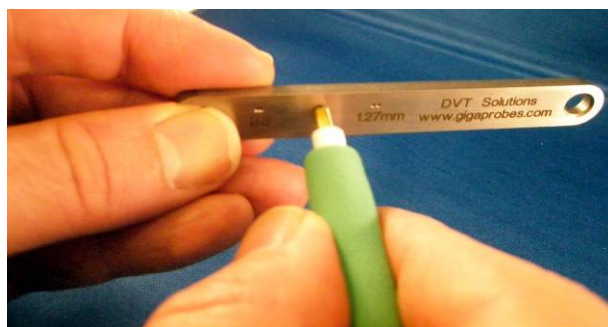
Fig. 3) Signal - Signal Pitch Calibration (patent pending) - Place the probe tips in the Model 10 SMA stainless steel calibration wrench adjusts S - S pitch to a fixed 0.8 mm, 1.0 mm. or 1.27 mm spacing. Use the Desk-Top Macro-lens Inspection Station to view probe tips, probing location and the precision Stainless Steel Tweezers for fine pitch adjustments.
