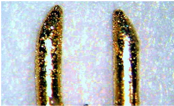
Fig. 4) Gold Plated Conductive Diamond Probe Tips (patent pending) – Hundreds of sharp, non-oxidizing, conductive diamonds on the probe tips break through surface oxide when probing, to create a connection equal to that of lead solder. Conductive Diamond technology improves repeatability of TDR measurements when probing at any angle.
