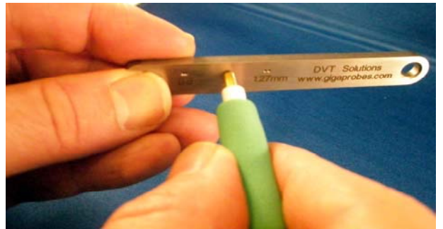
Fig. 3) Signal - Signal Pitch Calibration (patent pending) - Place the probe tips in the model 10 SMA calibration wrench to adjust S – S pitch to a fixed 0.8 mm, 1.0 mm. or 1.27 mm spacing. Use the Desk-Top Macro-lens Inspection Station to view probe tips and the precision Stainless Steel Tweezers for fine pitch adjustments.
