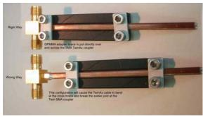
Install the GigaProbes in the GPMMA as demonstrated in the TOP picture with the twin SMA connector fully forward and the cross brace tightened along the top of the coupler
