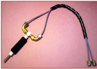
Fig. 1) 24 GHz Cables – 12" SMA to SMA 24 GHz cables are shown configured for manual probe operations.
