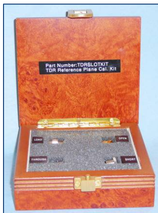
Fig. 5) DT Solutions LLC SLOT Kit – SMA Female connector, Short, Load, Open, Through, to calibrate measurement reference plane and subtract out cable loss
