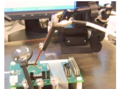
Use the 5x magnification lens, part of the GigaProbes Accessory kit to view the probe location.
