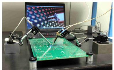
DVT-FP 100 flex manipulator (left) holding DVT-2MPUSB digital camera displaying FPGA pads of test board on Laptop. (Right) GigaProbes® TDR probes held in second DVT-FP100 manipulator probing pads viewed on laptop.
