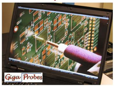
DVT-2MPUSB – Connect digital camera to your computer with USB cable to help view probing location and inspect small details, right on your computer screen!
