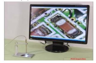
**DVT-2MPUSB** digital camera viewing SMT device to verify solder
